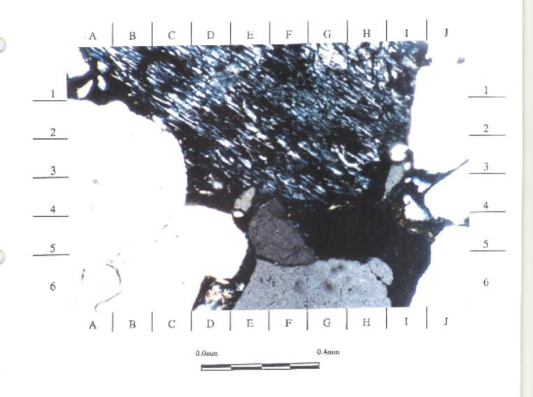
Figure 6. 1746.3m x75.6 XPL Quartz sandstone with heavily leached feldspar at E2. A detrital clay coating on primary pore space is also evident at J4.
