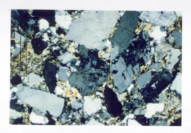
Figure 17, Anemone #1A, junk sub sample, 4676b m. Seen under crossed polars, the illitic matrix and sericitic grain replacements (Se) of the previous figure are obvious. The concentration of spar (S) is seen to coincide with an abundance of clay and may represent grain replacement.
