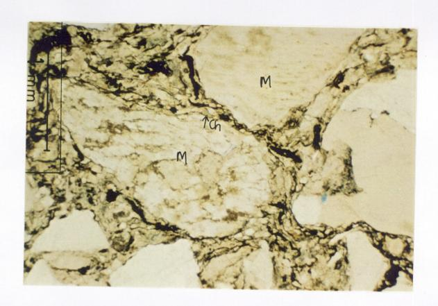
Figure 9 - Anemone #1A, junk sub sample, 4676a m. Thin section micrograph in plane polarized light showing alteration of microcline (M) and a plutonic fragment on the right. Stylolitic organic matter and fine pyrite pervade the matrix. A small lime green area of chlorite (Ch) is visible. Vague bluish areas in the matrix may be microporosity.
