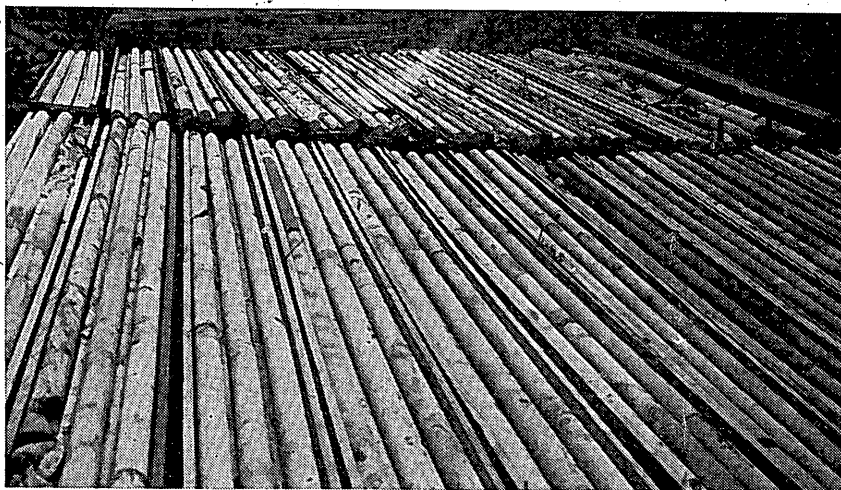
1000 feet of 2\frac{1}{8} -inch core from one horizontal well. Though the hole was level, note lateral variations in the sandstone—in texture and saturation. Note cross bedding planes.
