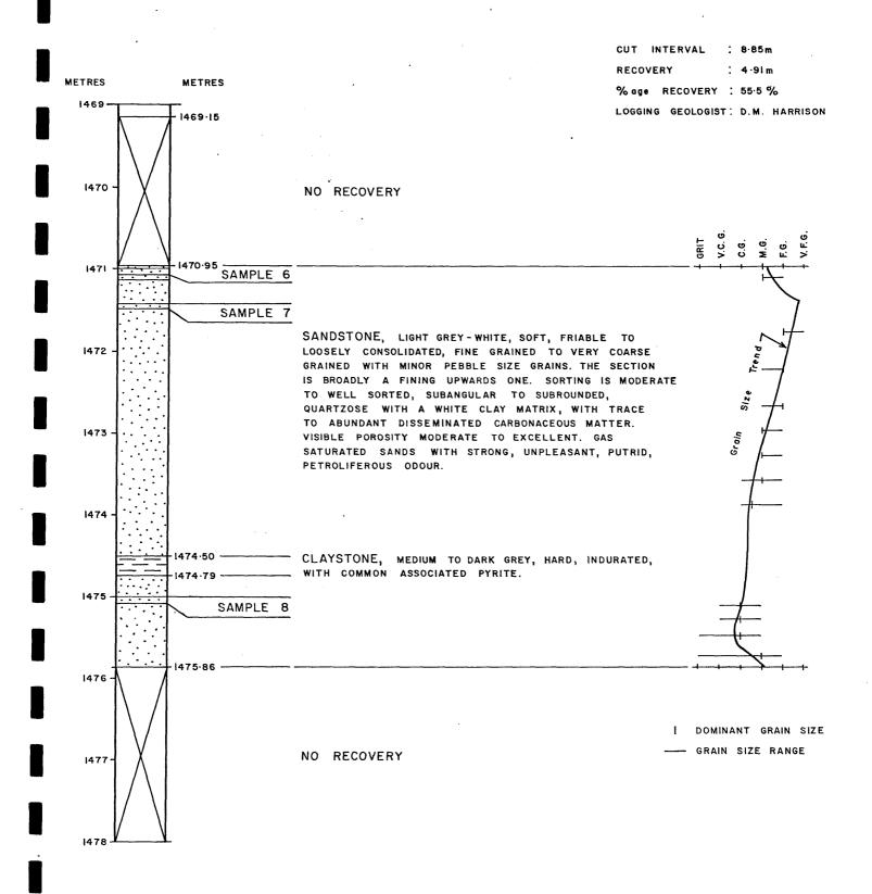
NOTE: THE SECTION WAS BASICALLY LOOSELY CONSOLIDATED AND FELL OUT OF THE CORE BARREL MINOR SECTIONS REMAINED INTACT AND CONSOLIDATED AT SURFACE. THESE WERE 1470-95 - 1471-13 m, 1471-4 - 1471-47, 1474-99 - 1475-16 m.
