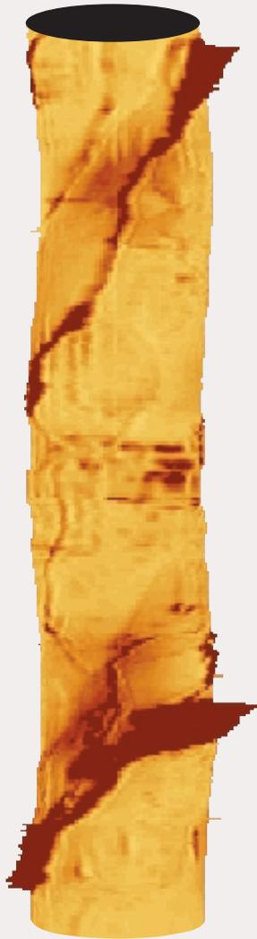
Formation image and dipmeter data are valuable sources of geological information relating to structures (folds, faults, unconformities and structural dips), to sedimentary geology (facies, bedform orientations and palaeocurrent directions) and to stress orientations (breakouts).
