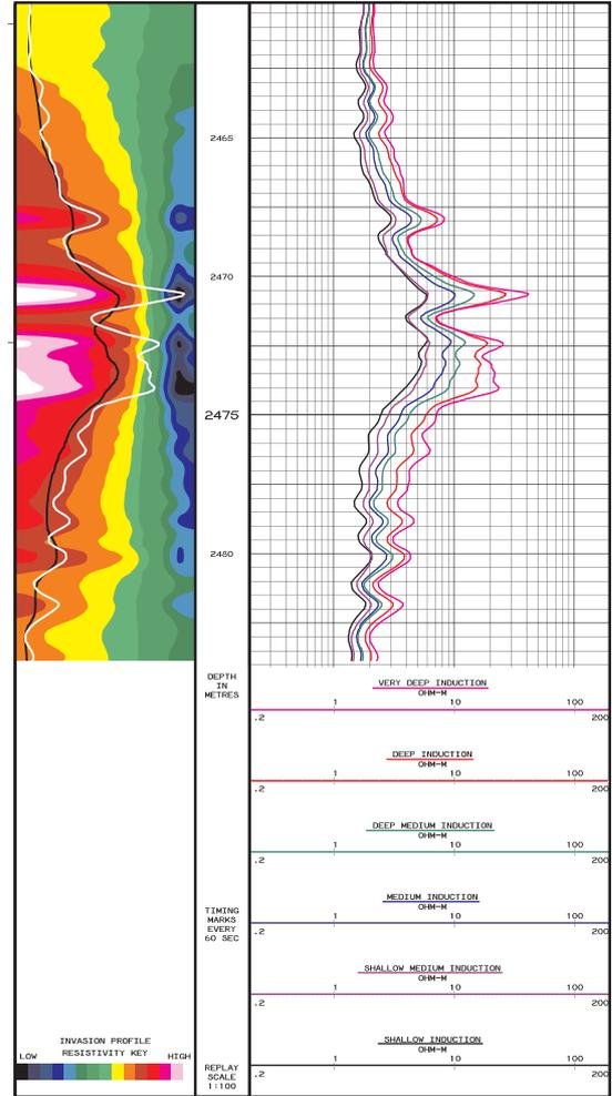
VECTAR<sup>®</sup> acquisition and processing enhances the resolution of many conventional logs by between 50 and 300 %, giving improved bed definition, core correlations and nett pay results in thinly bedded and complex reservoirs.
