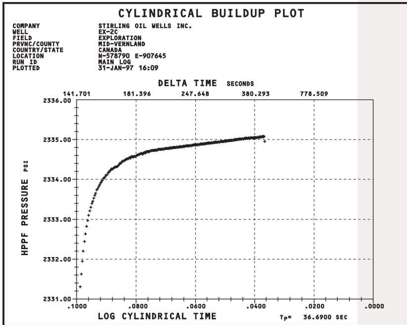
RFS pressure-time function plots are used to compute intrinsic formation pressures and to provide estimates of formation permeability. During acquisition, tests are terminated as soon as the computed formation pressures reach steady values - this can greatly reduce total logging times.
