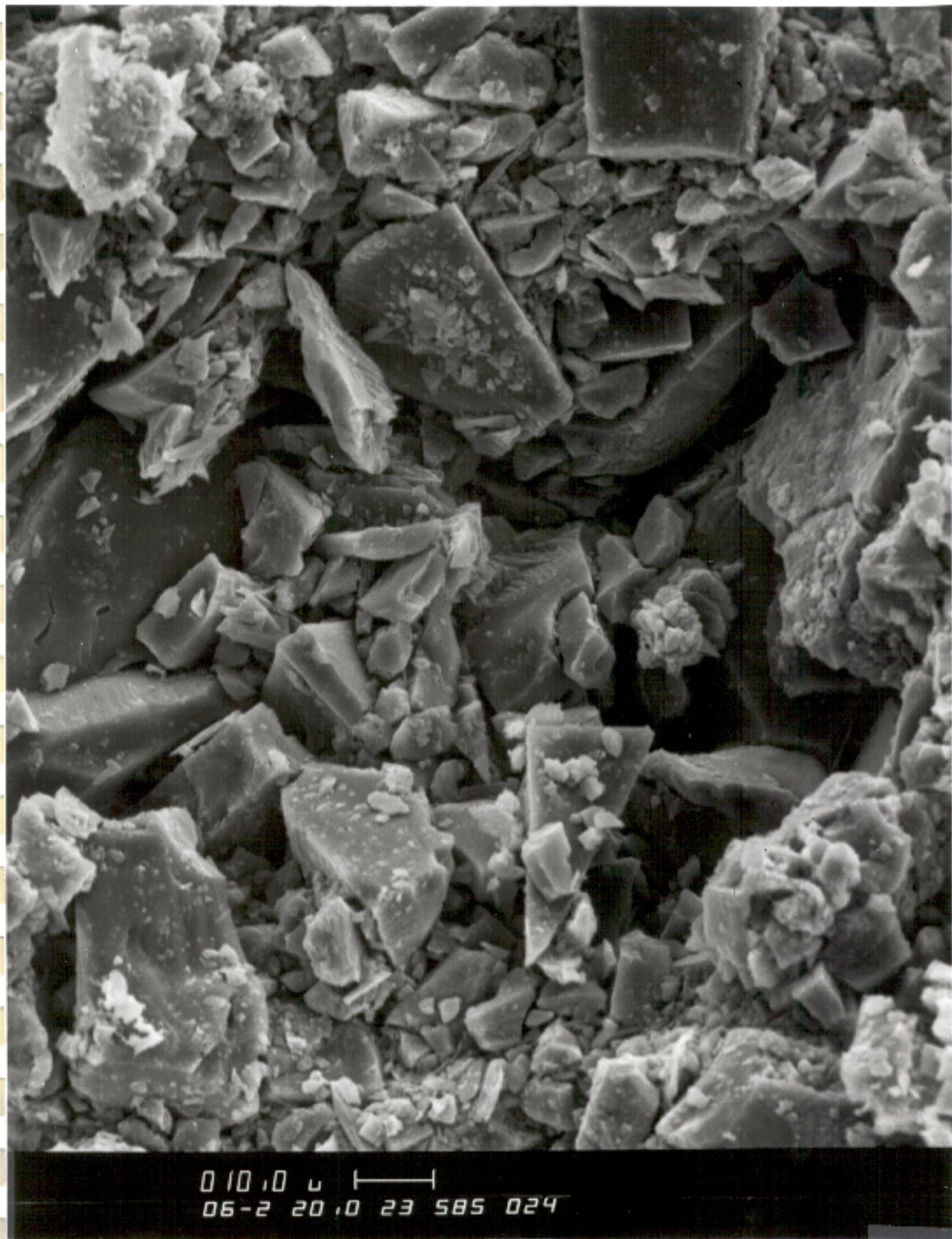
PLATE 6: 1491.5 m The fine-grained mineral matter consists largely of angular quartz cemented by allochthonous clays (kaolinite, illite and chlorite).
