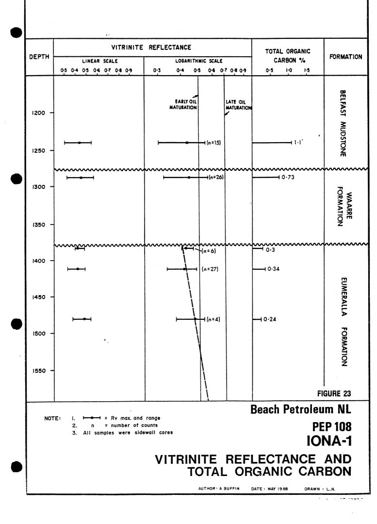
TOC content of the Waarre, Unit D was moderate to good and DOM matter common, inertinite was the common maceral, whilst vitrinite was sparse and exinite rare, reducing the source rock potential of the Waarre, Unit D. The vitrinite reflectance data and spore pollen colour confirms the Waarre, Unit D is immature for hydrocarbons.
