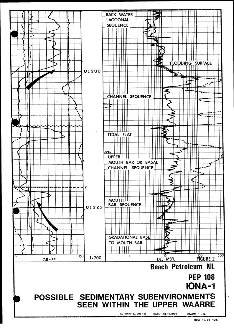
Unit A consists of a fining upward sequence with a high resistivity peak that may represent a thin limestone bed, overlying the Eumeralla uncomformity.
