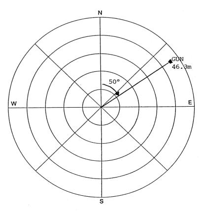
INDICATE GUN/VIBRO AND HYDROPHONE OFFSET AND AZIMUTH RELATIVE TO NORTH
