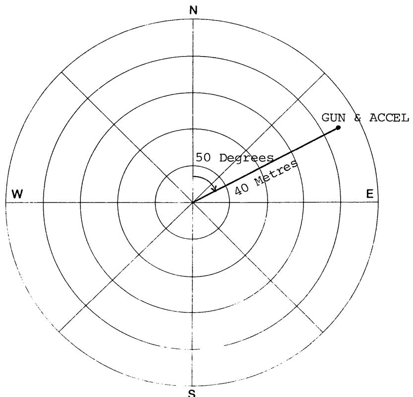
INDICATE GUN/VIBRO AND HYDROPHONE OFFSET AND AZIMUTH RELATIVE TO NORTH
