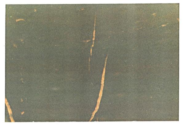
Plate 2: Same field as above Fluorescence Mode Exsudatinite and liptodetrinite have a moderate orange fluorescence whilst suberinite fluorescence is notably "dull".
