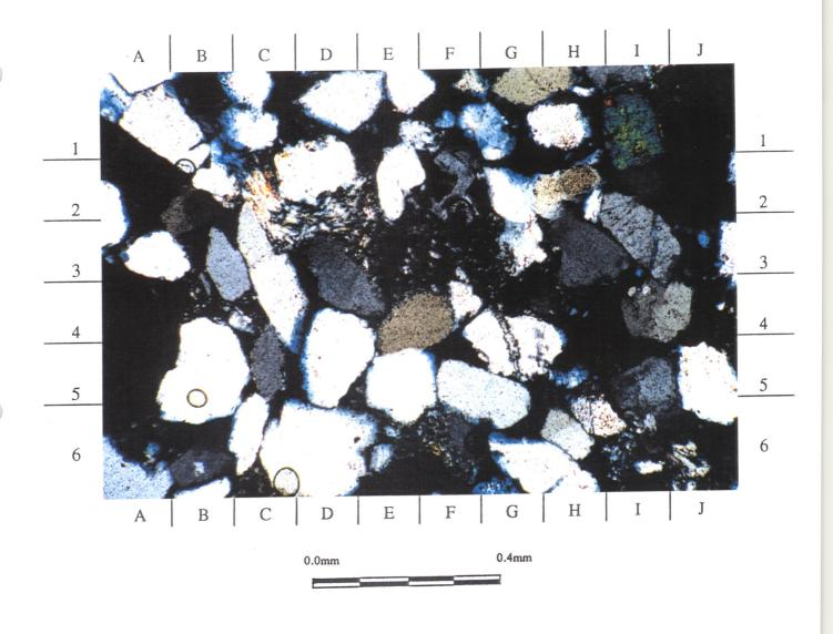
Figure 3. 1745.4m x75.6 XPL Quartz sandstone. A weak preferred alignment of the elongate axis of the detrital quartz is evident running from A1 to J1. A partially kaolinised muscovite grain can be seen at C2, with increasing kaolinisation to G3.
