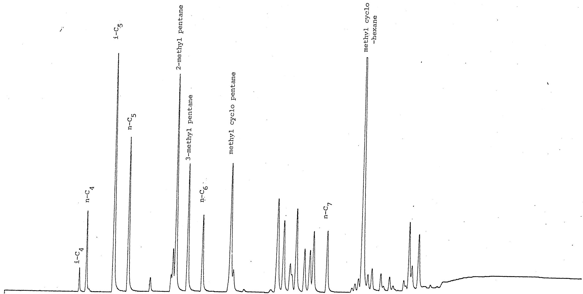
FIGURE 10 C<sub>4-7</sub> GASOLINE RANGE CHROMATOGRAM: RET NO. 4; 1387.7m, TARWHITE-1.
