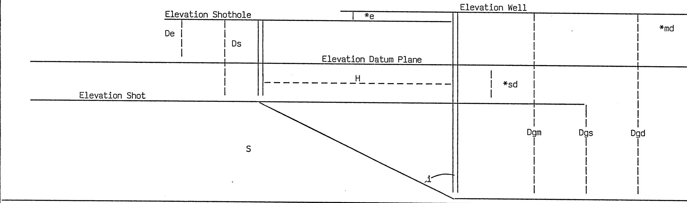
Dgm = Geophone depth measured from well elevation
