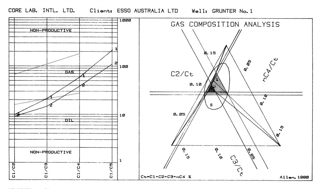
NO. DEPTH C1 C2 СЭ 1C4 nC4 C5 C6 % Ct C1/C2 C1/C3 C1/C4 C1/C5 1 3224 0.365 0.037 0.017 0.003 0.003 0.002 0.001 0.423 10 21 59 215 CONCLUSION: MODERATELY PERMEABLE GAS ZONE 2 3347 1.225 Ø. 137 0.084 0.016 0.016 0.011 0.006 1.462 9 15 38 109 CONCLUSION: WET GAS ZONE
