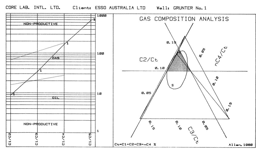
NO. DEPTH C1 C2 СЭ 1C4 nC4 C5 C6 % Ct C1/C2 C1/C3 C1/C4 C1/C5 1 3522 2.079 Ø. 239 0.081 Ø. ØØ6 0.008 0.003 0.002 2. 388 9 34 185 871 CONCLUSION: TIGHT. WET GAS ZONE
