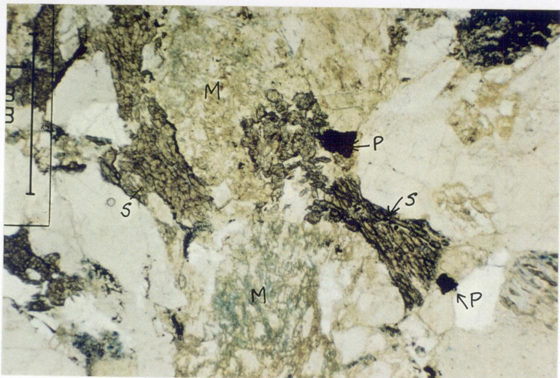
Figure 59 - Anemone #1A, junk sub sample, 4676f m. General view in plane polarized light showing secondary dissolution porosity associated with highly altered microcline (M). Aggregates of spar scalenohedra (S) and pyrite (P) are evident.
