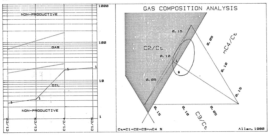
C1/C2 C1/C3 C1/C4 C1/C5 C5 C6 % СЗ 1C4 nC4 NO. DEPTH C1 C2 0. 309 3 19 21 1 2417 Ø. 180 0.008 Ø. ØØ8 Ø. Ø69 Ø. Ø55 0.005 CONCLUSION: LOW GOR OIL OR POSS. UNREPRESENTATIVE GAS SAMPLE
