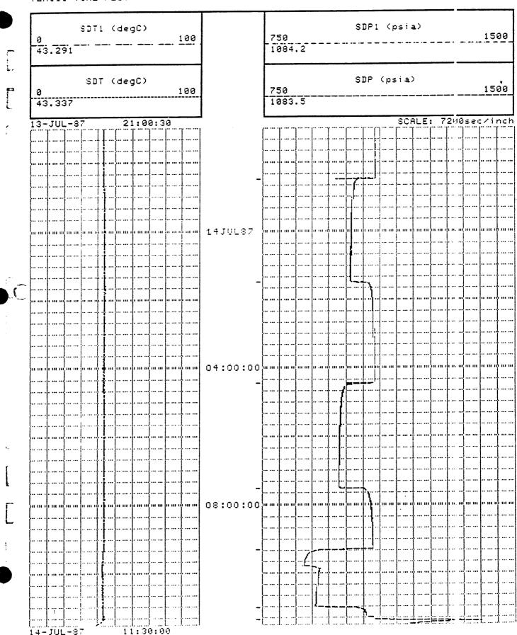
WELL TEST SDP BOTTOM HOLE REBULTS (linear plot) INITIAL FLOW , BUILD UP & CLEAN UP FLOW
